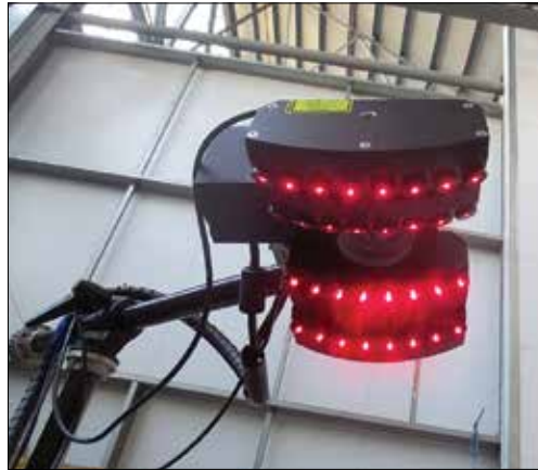
Equipment for performing laser shearography with dynamic excitation includes multiple piezoelectric transducers, far left , and larger laser illumination arrays, left .
