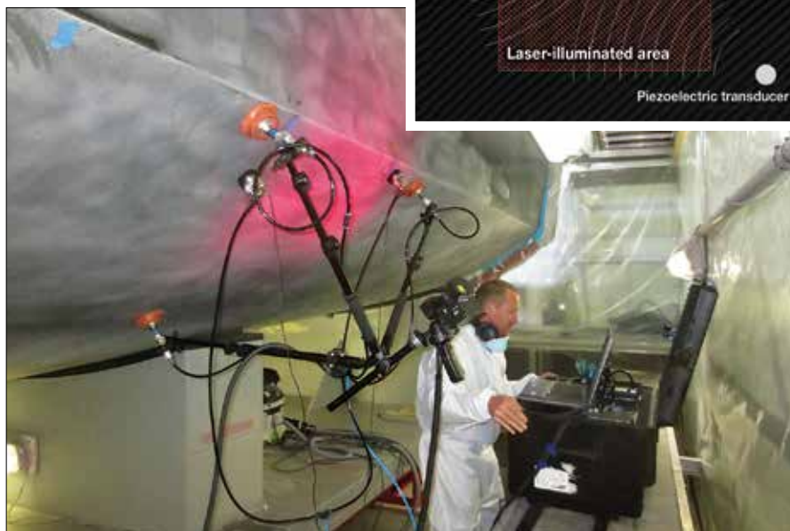
Expanded-FOV shearography utilizing dynamic excitation, rather than a vacuum, to stress the test surface can shoot a larger area (28" x 20"/70cm x 50cm), including complex forms such as chines. Inset —With this method, piezoelectric transducers send ultrasound waves through the structure at different frequencies to reveal discontinuities or defects, which resonate at frequencies different from those in the surrounding sound laminate.
