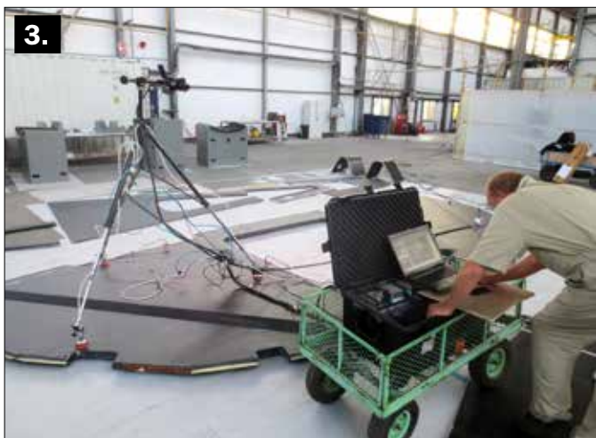
In just 30 hours, NDE technicians, working primarily at night so they wouldn't interfere with the build crew, inspected the complete 7,000-sq-ft (650m 2 ) composite surface area of a 100' high-performance sailing yacht. 1 —The project started with the inner skins of the hull and deck parts while they were still in their female tooling. 2 —Next, the outer skins were tested when the parts were released from the tooling. Note how far apart the two piezoelectric transducers (at the ends of the white cables) are on the hull surface. 3 —Bulkheads were inspected flat on the shop floor before installation. 4 —Here, the curved hull bottom is bathed in red laser light during testing. The full project revealed mostly common defects in bondlines between prepregs and the Kevlar core. The tests enabled the builder to correct those flaws before the vessel went into service.
