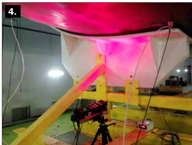
In just 30 hours, NDE technicians, working primarily at night so they wouldn't interfere with the build crew, inspected the complete 7,000-sq-ft (650m 2 ) composite surface area of a 100' high-performance sailing yacht. 1 —The project started with the inner skins of the hull and deck parts while they were still in their female tooling. 2 —Next, the outer skins were tested when the parts were released from the tooling. Note how far apart the two piezoelectric transducers (at the ends of the white cables) are on the hull surface. 3 —Bulkheads were inspected flat on the shop floor before installation. 4 —Here, the curved hull bottom is bathed in red laser light during testing. The full project revealed mostly common defects in bondlines between prepregs and the Kevlar core. The tests enabled the builder to correct those flaws before the vessel went into service.
