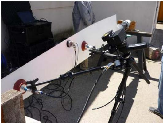
Shearography equipment attached to the rudder
