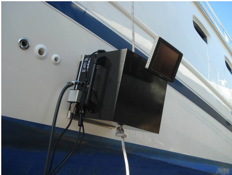
The vacuum hood attached to the side of the GRP production motor yacht
