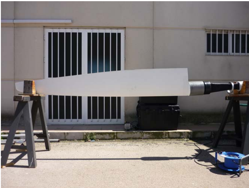
Rudder-blade removed and placed over trestles for the inspection.
