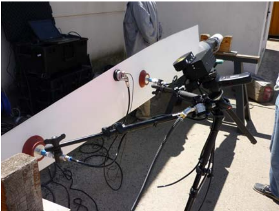
Shearography equipment attached to the rudder
